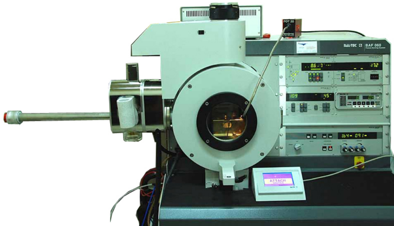
The BAF 060: fracture and coat for cryo-SEM, or prepare freeze-fracture replicas (FFR)
