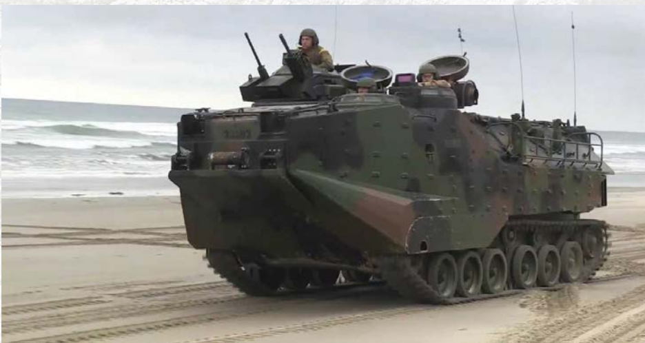
Figure 1. The AAV-7 amphibious assault vehicle in action. “Designed to assault any shoreline from the well decks of Navy assault ships, AAVs are highly mobile tracked and armored amphibious vehicles that transport Marines and cargo to and through hostile territory.” Photo at www.marines.com/operating-forces/equipment/vehicles/aav-7#features .
