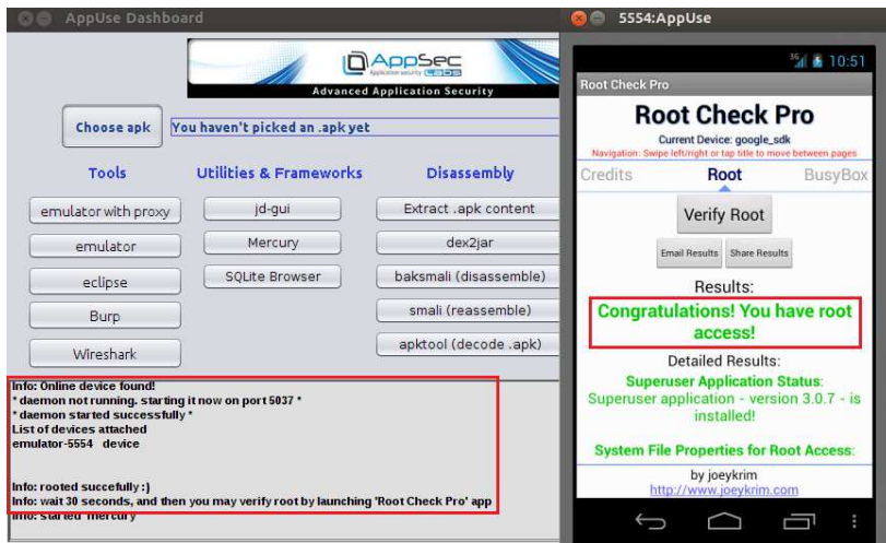
Figure 10 - The results from Root Check Pro application – successfully rooted the emulator with a click.
