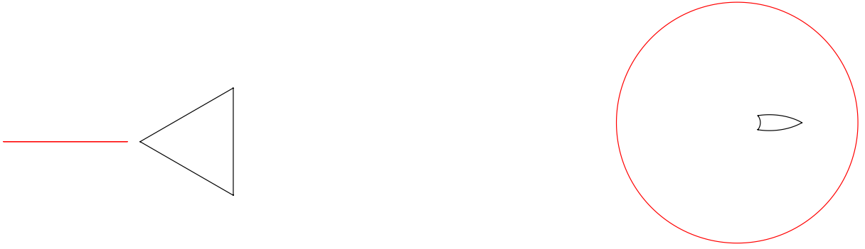
FIGURE 16. The segment and polygon domain \Omega for a = 1.6 and r = 0.5 (left); and the image of this unbounded domain under the mapping \zeta = \Psi^{-1}(z) (right).
