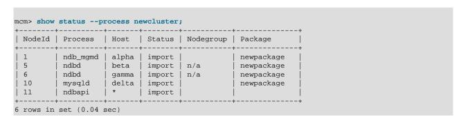
Having the import status causes any of the commands start cluster, restart cluster, start process, and stop process to fail if they are executed before an import cluster command has been executed against this cluster. It is also not possible to execute upgrade cluster on a cluster having processes with import status. Other operations on this cluster continue to be performed normally.
