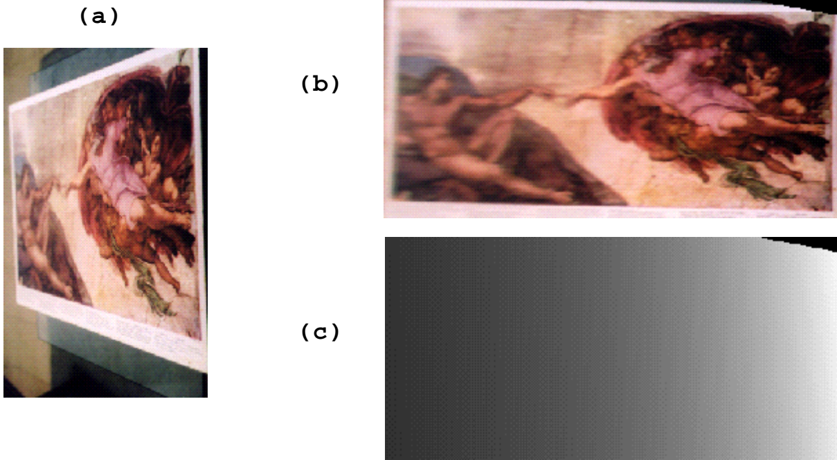
Figure 12: Second original image (a), its mapping into a rectangular texture space (b), and the certainty map of the mapping (c).
