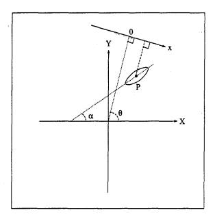
Fig. 1. Coordinate systems of the 2D plane and measurement projection line.  $\theta$  is the projection angle and  $\alpha$  is the angle by which the axes are rotated.
