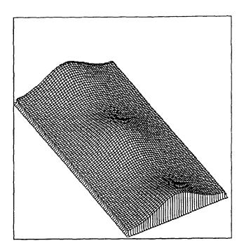
Fig. 4. Surface of predicted trace( $\Sigma_F$ )<sub>t+1</sub> as a function of the projection plane orientation.
