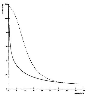
Fig. 5. Results of a comparisson between the active and passive methods. The horizontal axis presents the number of projections taken by the two methods. The vertical axis measures the uncertainty  $(trace(\Sigma))$  corresponding to the estimated positioning of the feature. The dashed line presents the passive results while the solid line presents the active method results.
