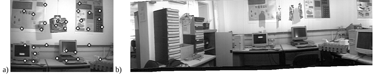
FIG. 3. Mosaicing examples. a) Point selected for motion computation. Four of the thirty points are located on the moving pendulum. b) Panoramic image that was created while a pendulum was swinging. The alignment was not affected by the outliers.
