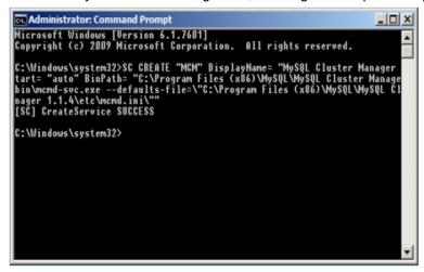
In addition, you should keep in mind that the spaces after the equals signs following the DisplayName, Start, and BinPath arguments are required.
