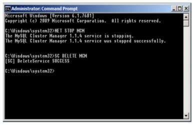
If the service is running at the time that SC DELETE is executed, the removal of the service takes effect the next time the service is stopped. In such a case, you must stop the previous instance of the service manually, and allow it to be removed, before you can reinstall the service.
