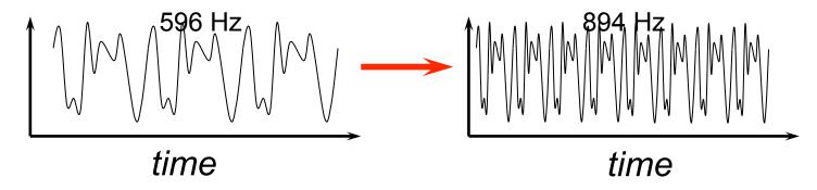
However, for most pitch shifts, integer increments (and memory pointers) are not adequate
