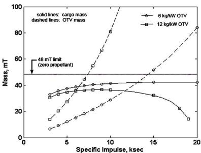
Figure 4: Effect of specific mass  $(\alpha)$  on cargo system performance. Transit time is 180 days.
