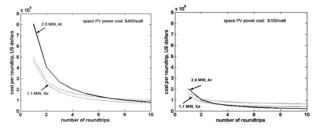
Figure 5: Cost dependence of lunar cargo technologies on propellant cost, power cost and system lifetime.
