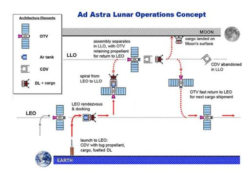
**Figure 1. Architecture of Lunar Cargo System.** The solar-powered VASIMR<sup>TM</sup> OTV (orbital transfer vehicle) is launched to low Earth orbit, followed by launch of a CDV (cargo delivery vehicle) for each round trip to low lunar orbit and back.
