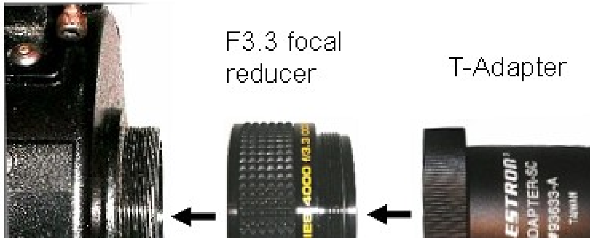
Figure G-4. Video camera adapted to telescope with f.3 focal reducer and T-adapter.
